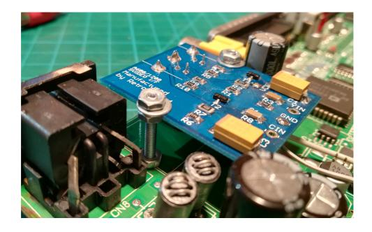
Solder wires from PIN 15 of CXA1145 chip to CIN and PIN 16 of CXA1145 to YIN on S-Video PCB.
