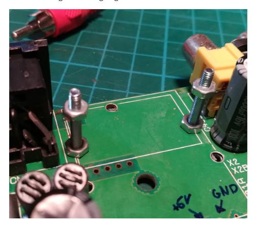
Solder GND and +5V wires to Amiga PCB
