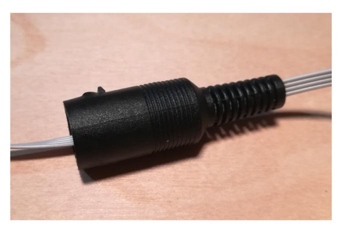
3. Solder all wires to a DIN6 plug according to wiring diagram and secure pins with shrink wrap.
