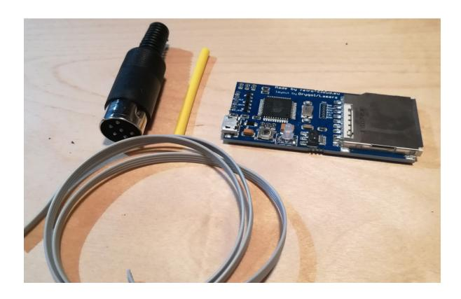
In order to connect SD2IEC do a DIN6 plug, you will need four wires. Four wires should be soldered to SD2IEC PCB on the one end  $\rightarrow$  CLK, DAT, ATN, GND and on the other end to a DIN6 plug.
